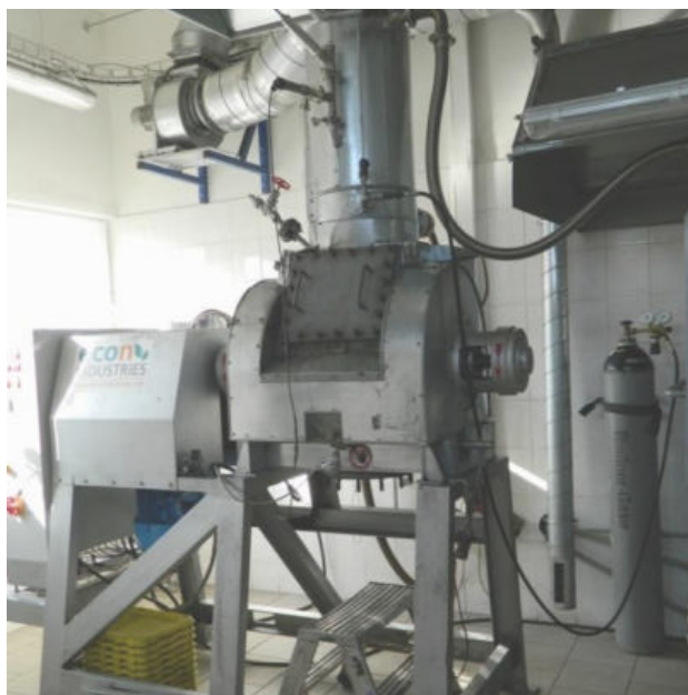
Fig. 2. Mixed dryer of semi-pilot testing unit.
