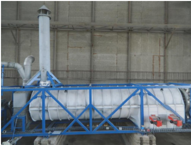
Fig. 4. Rotary kiln of continuous thermal desorption pilot unit.
