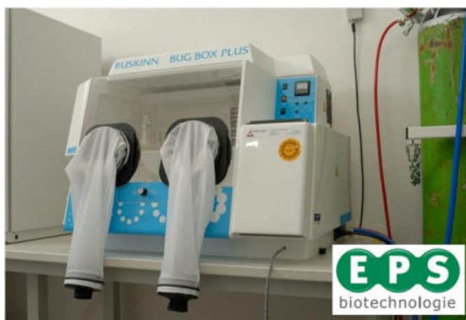
Fig. 1. The key device in environmental microbiology – glovebox for anaerobic manipulation with microorganisms (laboratory of EPS in Kunovice)
