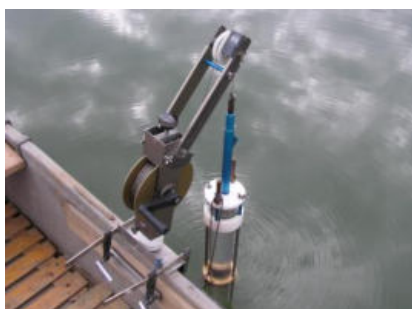
Fig. 1. Sediment sampling device (UWITEC).
